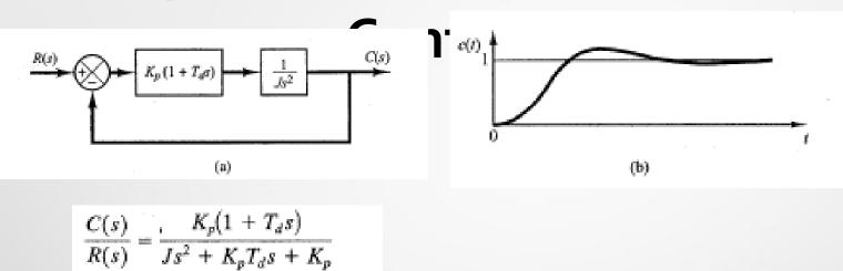
. Thus derivative control introduces a damping effect. A typical response curve *c* (*t*) to *a unit step* input is shown in
