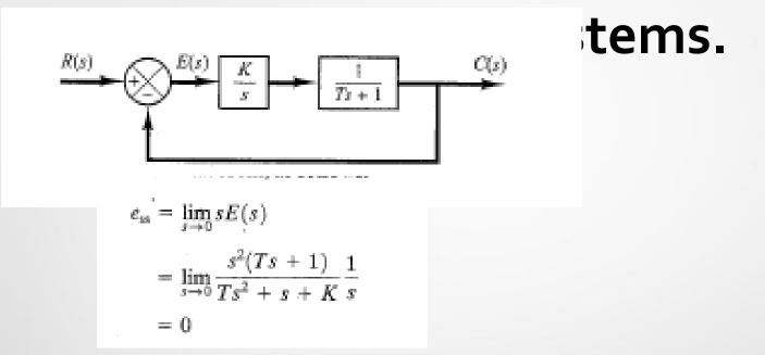
Integral control of the system eliminates the steady-state error in the response to the step input..
